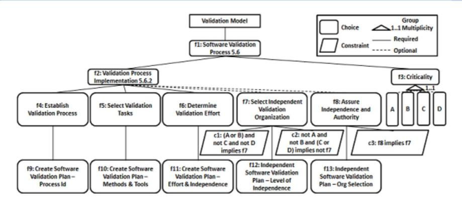
As we had 6 common elements, **SoC computes to 6**. We have at least 4 single processes. The number of elements in the single processes for criticality levels A, B, C and D are 10 (f4 through f13), 10 (f4 through f13), 6 (f4, f5, f6, f9, f10 and f11) and 6 (f4, f5, f6, f9, f10 and f11) respectively. Thus, **PrR's for single processes A, B, C and D are computed as 0.6, 0.6, 1 and 1 respectively**.
